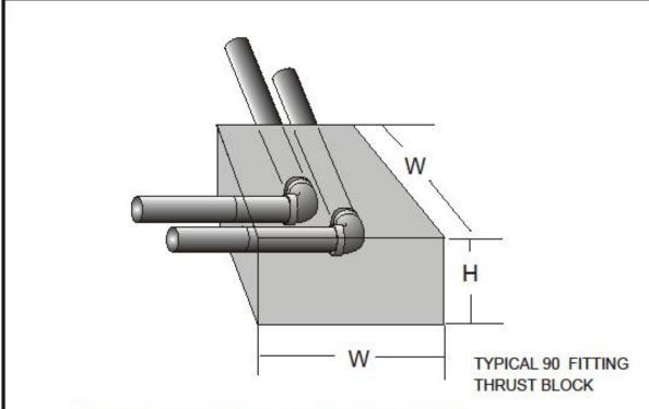
SQUARE FEET ON FACE OF THRUST BLOCK "F" TO BE PLACED AGAINST NATIVE SOIL CALULATED AS F sqft = H ftx W ft. DETERMINE TOTAL F IF MULTIPLE PIPE SYSTEMUSING:
